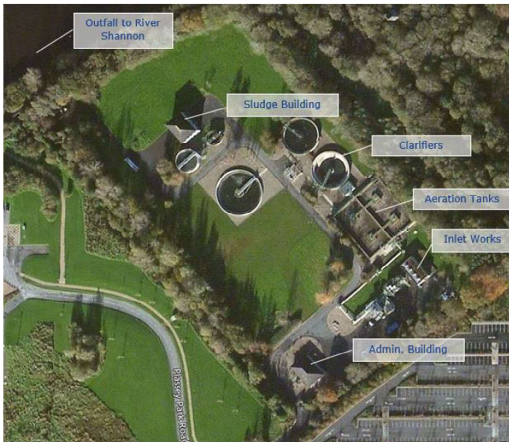
Figure 1-3: Castletroy WwTP Existing Layout
